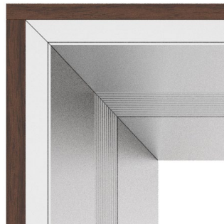
RIGHT Aluminum extrusion miter detail
